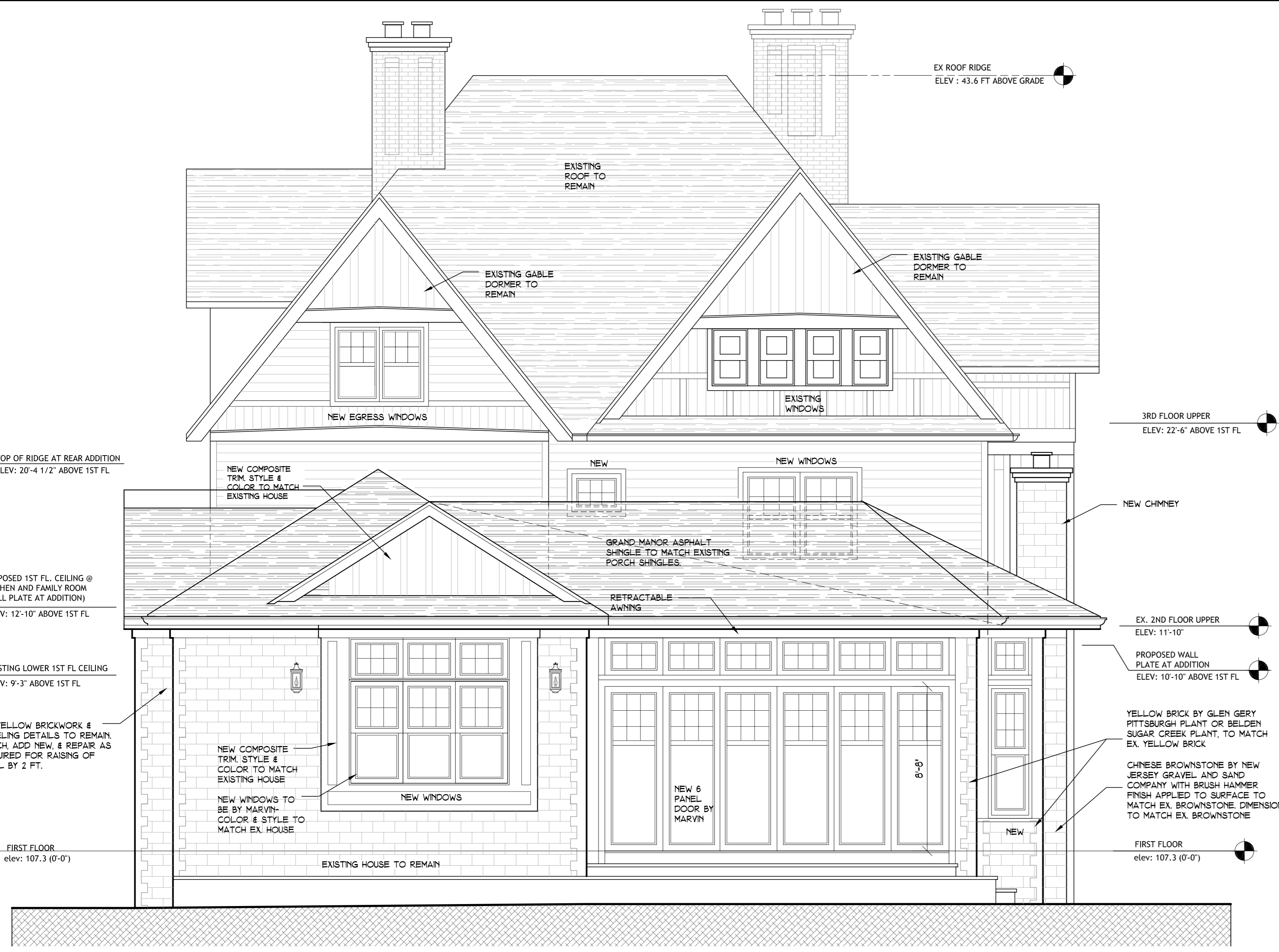
1 PROPOSED REAR ELEVATION (OPPOSITE IVY) A-05 SCALE: 1/4" = 1'-0"
